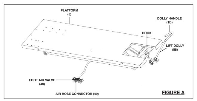
3. Once the Motorcycle Lift is unpacked, use the accessory Lift Dolly (58) to move the Lift to the desired assembly location. To do so, insert the Hook on the Lift's bottom chassis into the hole at the bottom of the Lift Dolly. Press down on the Dolly Handle (1D) to slightly raise the end of the Motorcycle Lift. Then, move the Lift to the desired assembly location. (See Figure A.)
